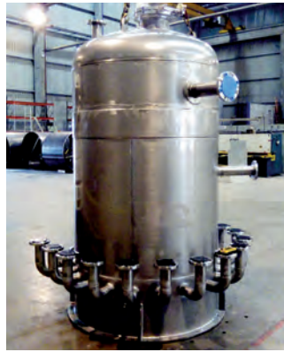
Foul Drain Seal Tank
