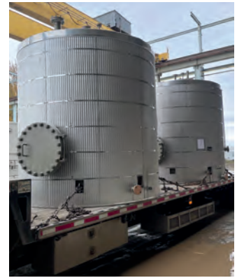
Sulphur Melter & Molten Tanks
